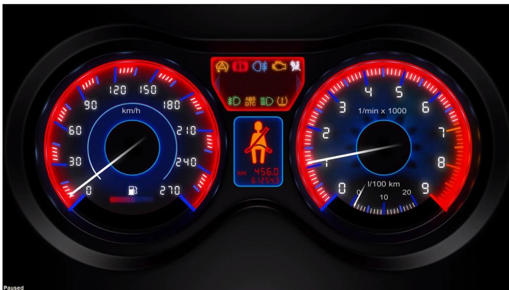
When the car starts and the accelerator is pressed the car is going nowhere as indicated by the speedometer on the left. But the tachometer on the right shows that the engine is working very hard. When the car does begin to move, the tachometer is always showing how hard the engine is working regardless of the speed.
